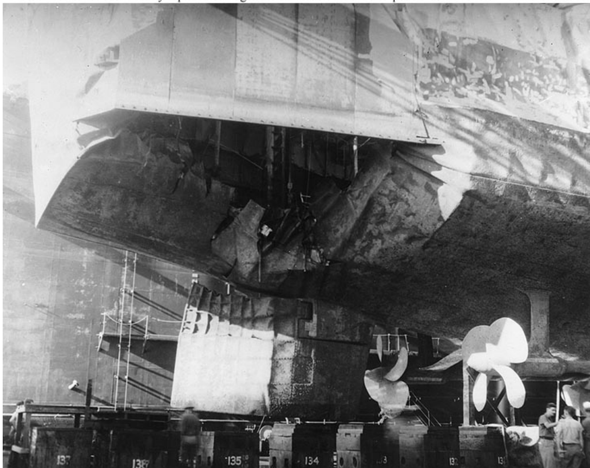
Photo # 19-N-105833 Partly repaired damage to USS Houston from a torpedo that hit her stern on 16 Oct. 1944
