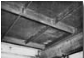
Photo 91: VIBURNUM (AN 57) Attachment of longitudinal girder to transverse lower deck beam end bulkhead B.
