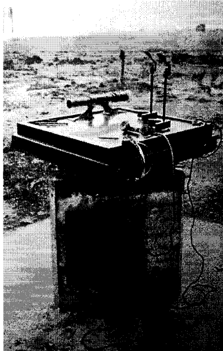
Figure 2.3. The mirror position finder, which was used to track the location of anti-aircraft shell bursts. Source: War Office, Text Book of Anti-Aircraft Gunnery , Vol. 1 (London: HMSO, 1925); copy available in AVHL I 1/33.
