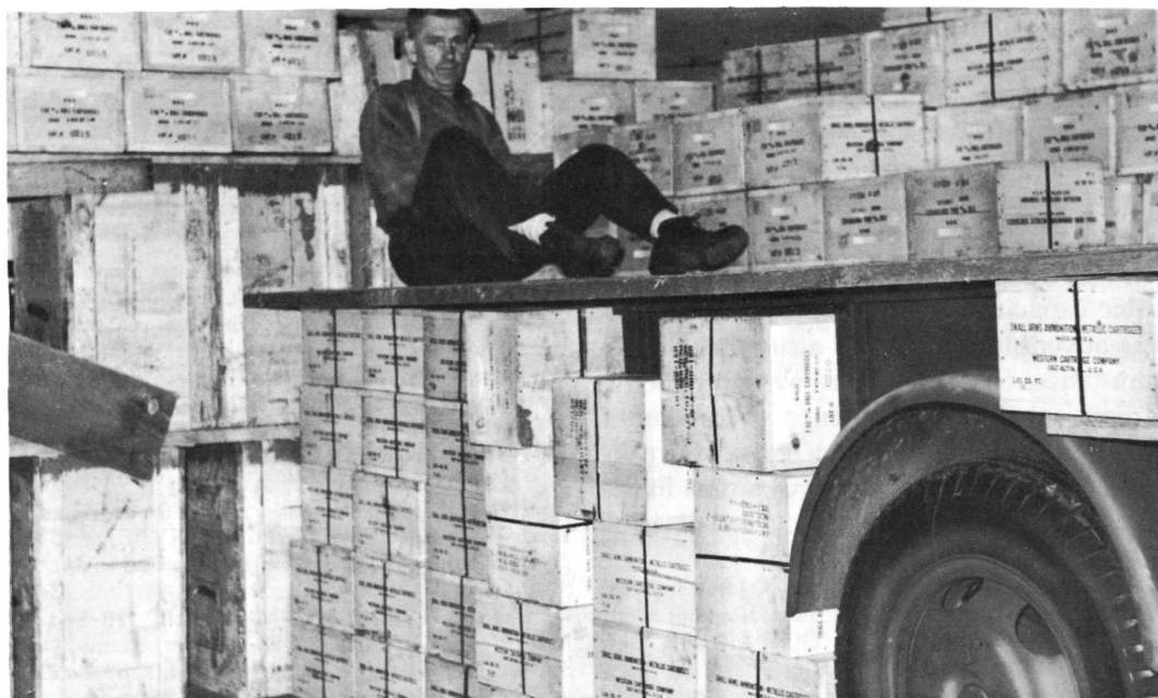
TIGHT STOWAGE OF PACKAGED FREIGHT in and around vehicles was employed to reduce loss of cargo space in shipping assembled trucks.
