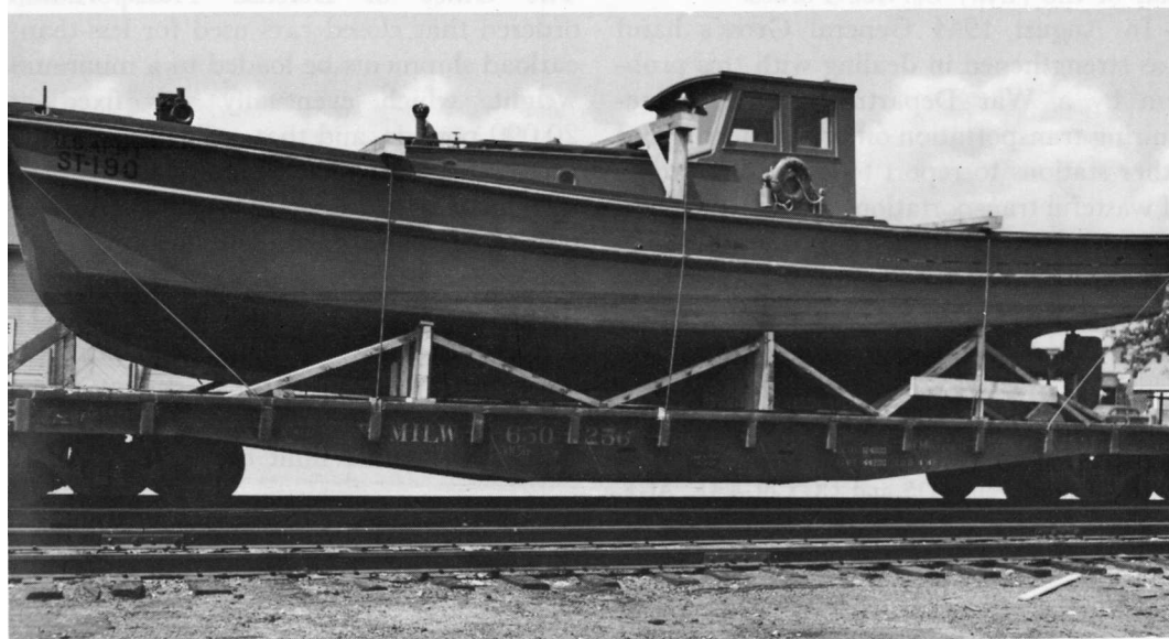
THE BRACING AND LASHING OF LARGE EQUIPMENT was carefully studied by the Transportation Corps and the railroads in order to facilitate handling and at the same time insure safe transit.
