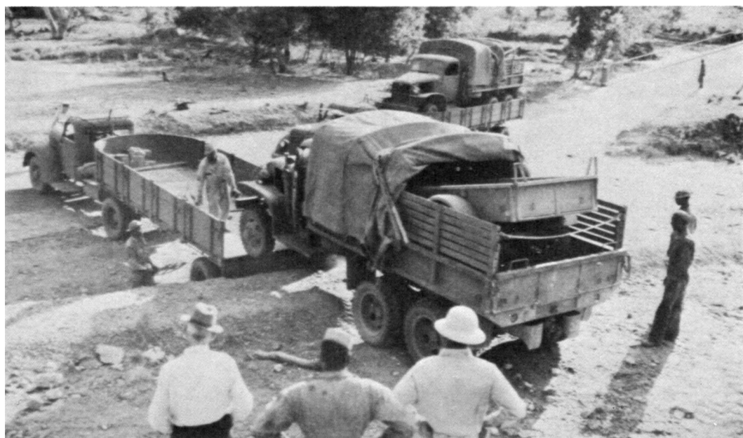
INGENIOUS USE OF TERRAIN FEATURES by individual units facilitated the delivery of supplies and equipment. The gravel bed of a stream used as a road when equipment bogged down in the tundra on Attu (above), and a roadside bank used as a loading ramp in Australia (below).
