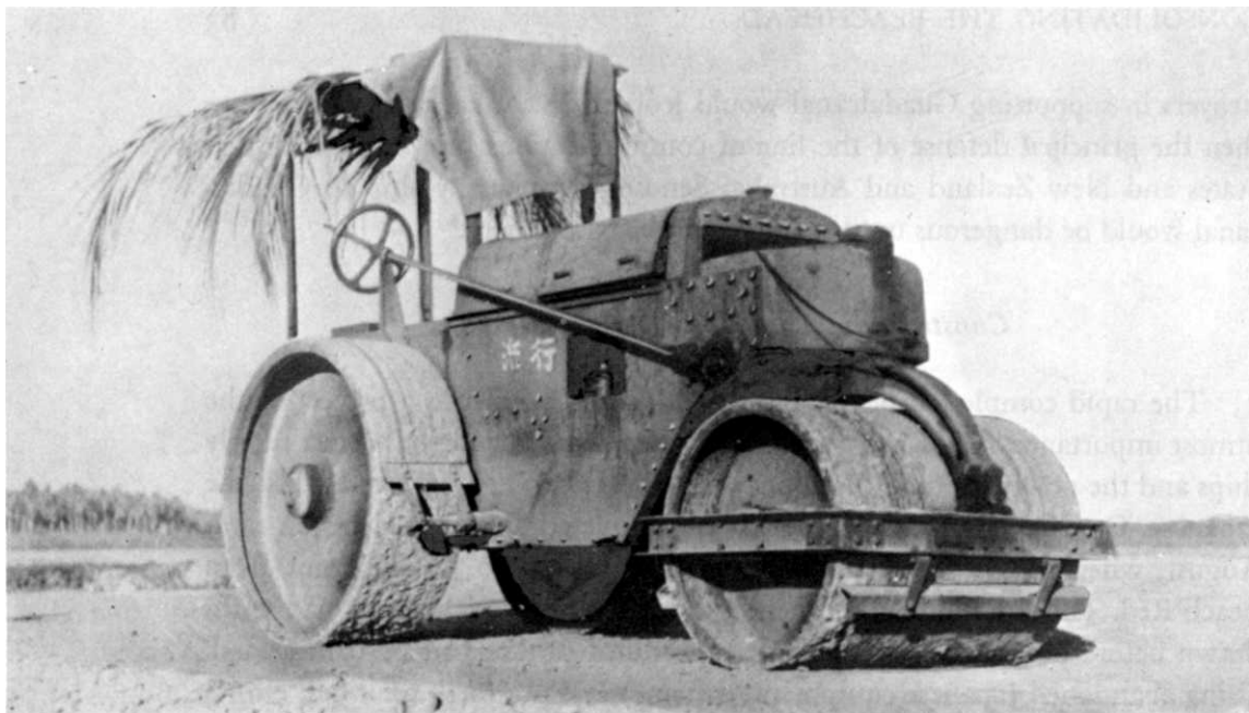
IMPROVING THE LUNGA AIRFIELD. Engineers used this Japanese roller to complete the half finished runway shown in the lower photo, taken shortly after the Marines landed on Guadalcanal. Note the profusion of bomb holes.
