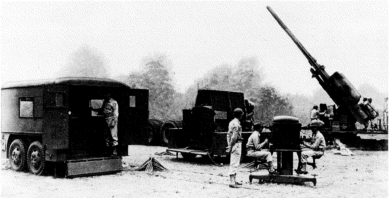
Figure 10. M-9 gun director in action. The tracking unit with its two operators is in the foreground, while the computing units are in the truck.
